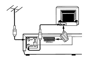
Remove the aerial cable from your TV set and plug it into the socket TF at the back of the video recorder.
